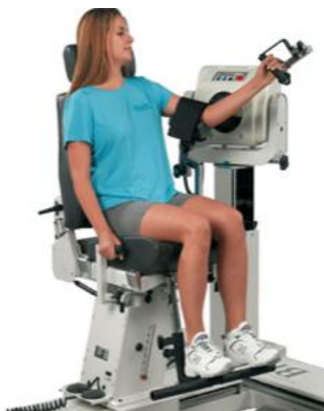
Fig. 3. Elbow-flexion test on Biodex System 3 dynamometer
