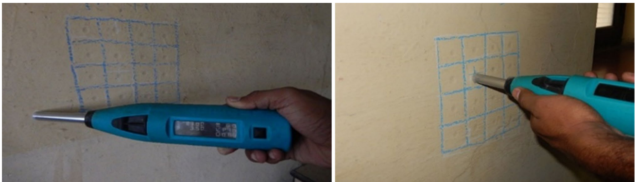
Fig. 4 Schematic view of the Schmidt Rebound Hammer
