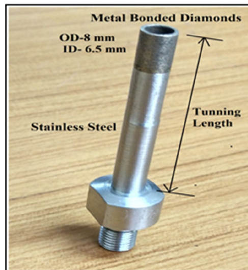
Figure 5. Photographic view of fabricated metal bonded diamond core drill picture.
