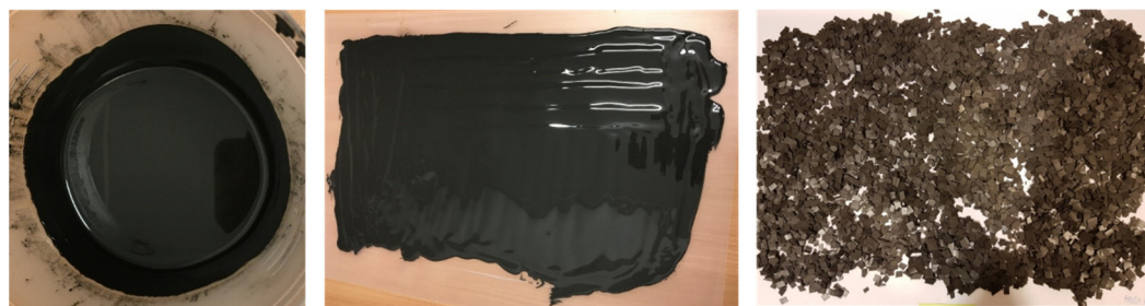
Figure 4. Composites at subsequent stages of fabrication: mixture of polymer, solvent and nickel powder after stirring (left), slurry after pouring on the foil (middle), final composite cut into granules (right).
