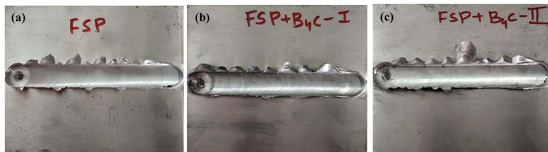
Figure 2. Surface modification of AA6061 (a) only FSP, (b) with B 4 C single pass and (c) with B 4 C dual-pass.
