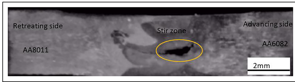
Figure 4. Macrostructure of friction stir welded joint (higher strength specimen).
