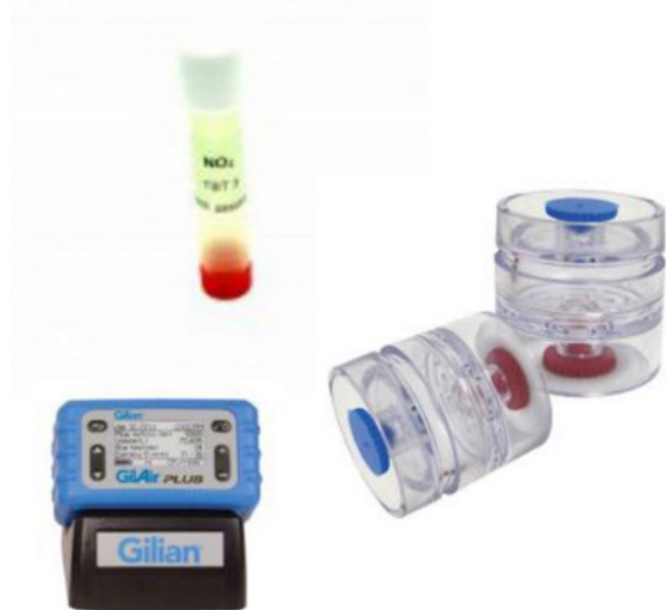
Fig. 2. NO 2 and PM 2.5 sampling devices
