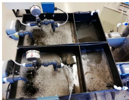
Figure 5. The MBR unit with a membrane compartment and an SNaD during inoculation.
