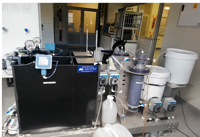
Figure 1. Poultry slaughterhouse wastewater (PSW) miniaturized lab-scale plant setup.
