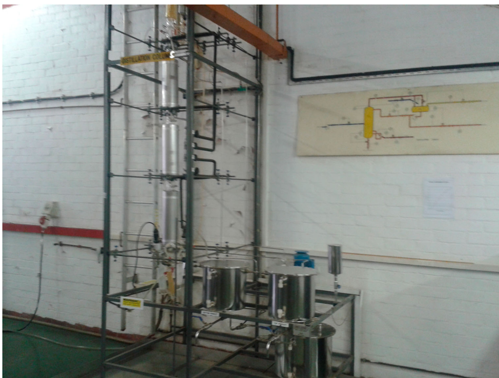
Figure 2. Bomikazi's chemical engineering laboratory; an actual distillation column, alongside a scientific drawing of a distillation column.
