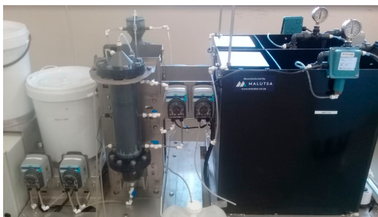
Figure 1. Photograph of the modified down-flow expanded granular bed reactor (DEGBR) (source: D.N. Dlamini).
