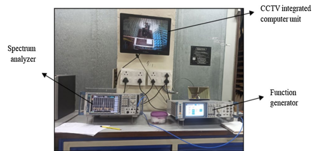
Fig. 16 Testing environment of the proposed antenna.
