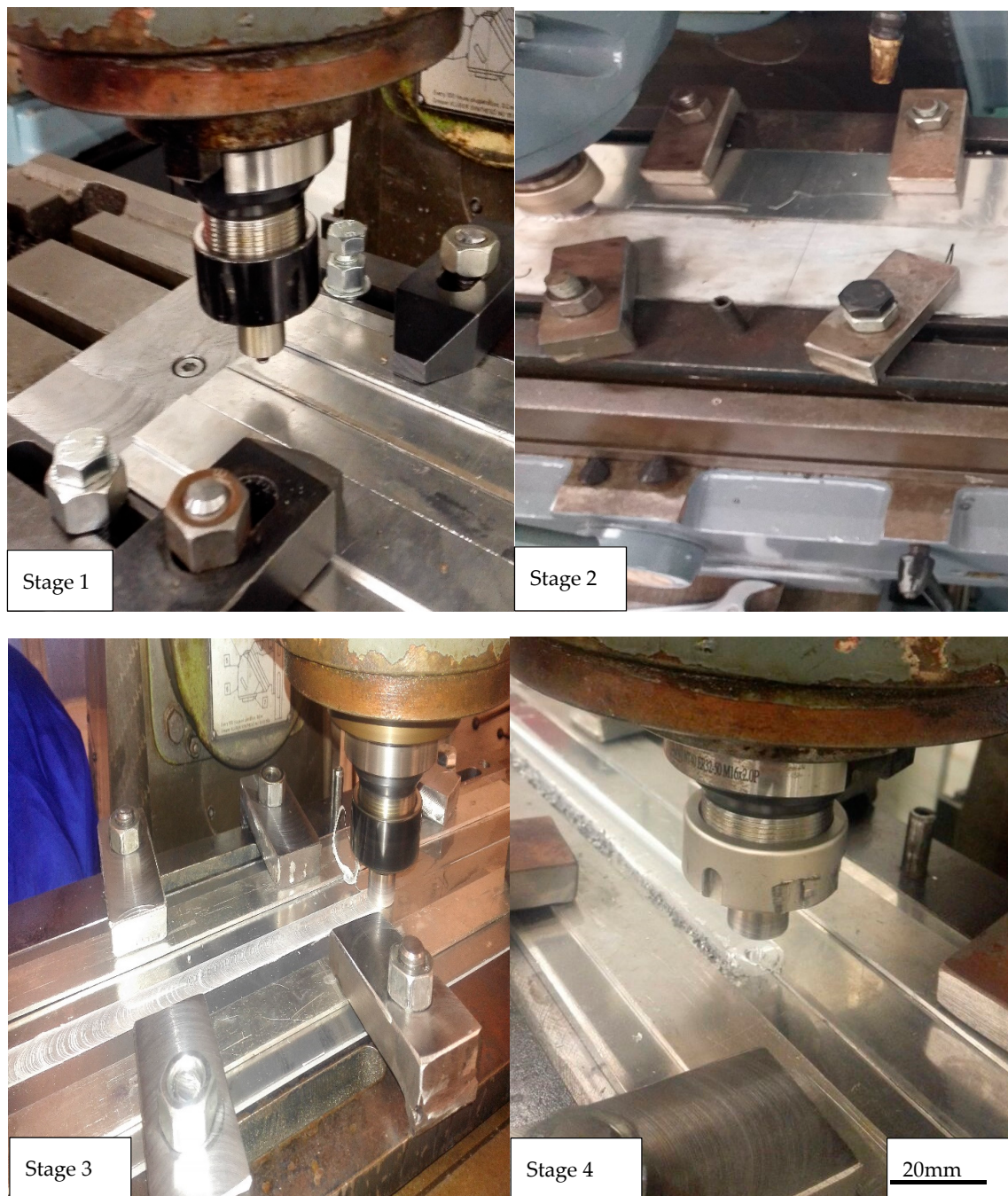
Figure 4. Friction stir welding process.
