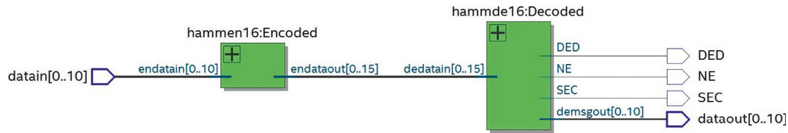
FIGURE 10: I/O overview of VHDL code for Hamming [16, 11, 4]_2 .
