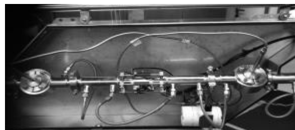
Figure 2: The industrially approved sensor unit featuring the unique custom made non-invasive transducer assembly.
