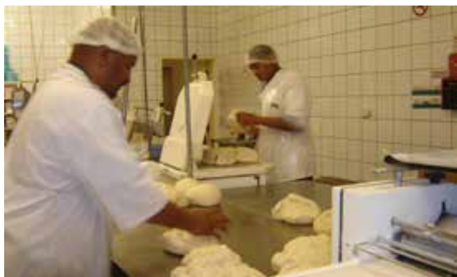
Fig. 2. Example of activity to reduce airborne flour dust exposures using divider oil (left) instead of flour (right) to prevent adhesion of dough to work surface.
