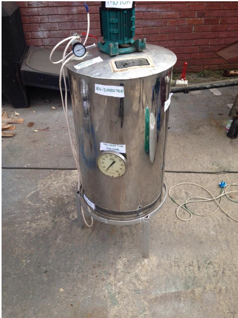
Figure 3: Prototype of the designed bio-digester A summary of the batch type bio-digester design considerations is given in Table 1.
