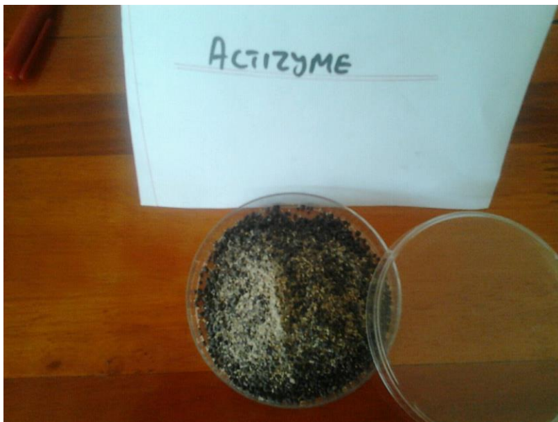
Figure 1: Acti-zyme a bio-catalyst used in anaerobic sewage digestion
