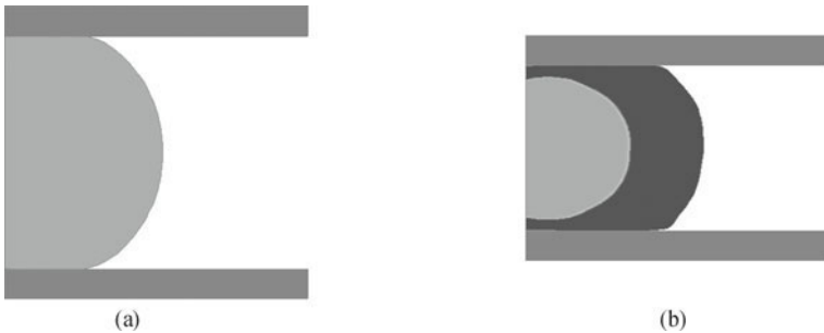
Fig. 2.6 Deformation of the cell model under force F = 3 \times 10^{-8} N: (a) hyperelastic cell, (b) liquid crystal cell with a hyperelastic nucleus.
