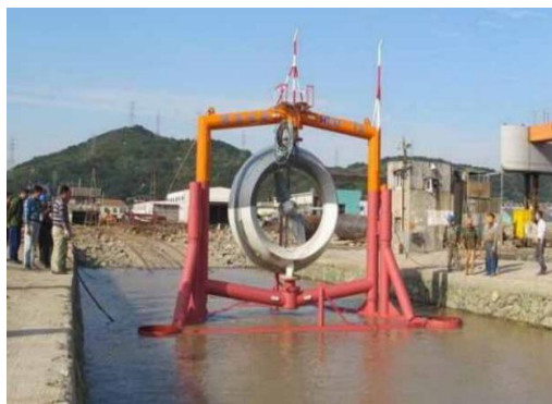
Figure 28. Haiming I: 10 kW submarine vertical-axis TCPG [112].
