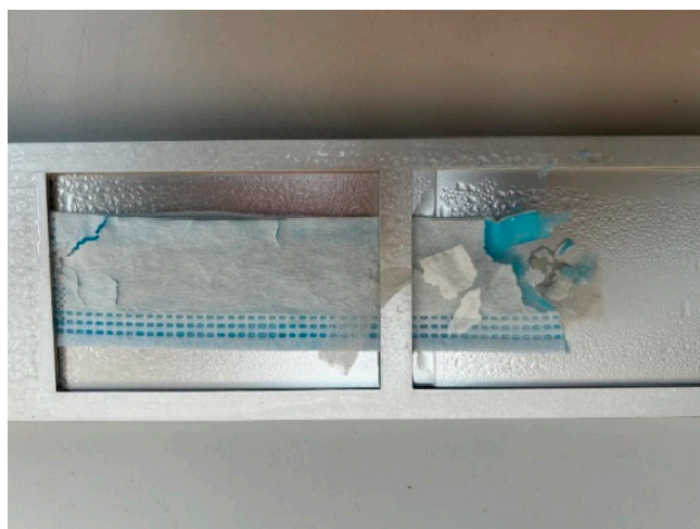
Figure 3. PP surgical mask after 120 h of exposure in the weathering test chamber.
