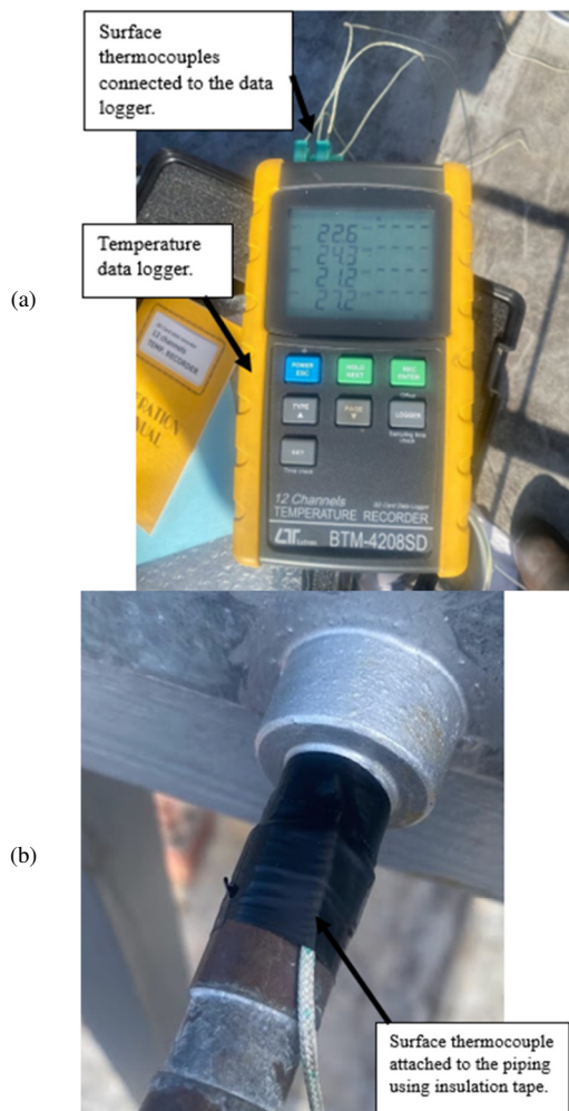
Fig. 4. (a) The temperature data logger, (b) surface thermocouple.
