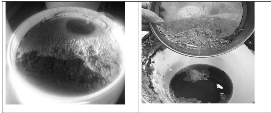
Fig. 3 a Aerobic pre-treatment of Eco-Flush™ enzymes and poultry slaughterhouse wastewater (PSW); b Filtration of feathers and suspended solids from PSW during the pre-treatment process
