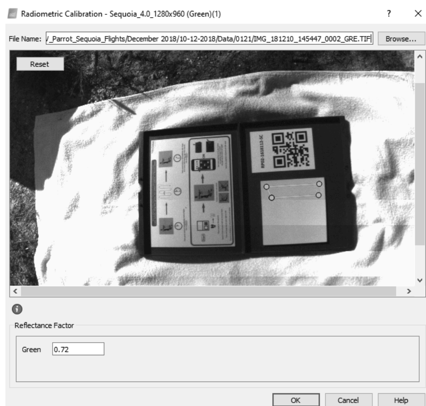
Figure 4. Application of reflectance factors on the green band calibration photos. The digitised rectangle denotes the area showing the reflectance in the green band. The value 0.72 is the reflectance factor.
