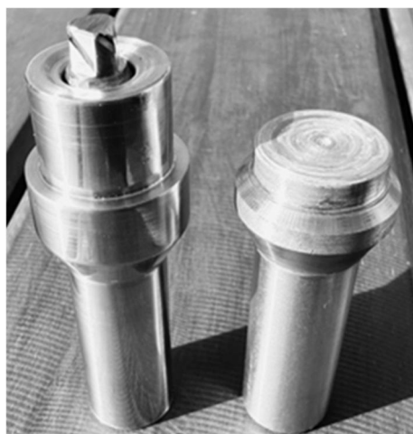
Figure 2. The tools with and without pins utilized in the composite production process.
