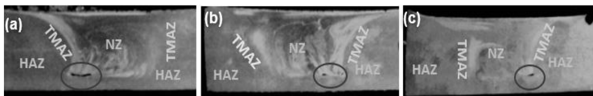
Figure 5. Macrographs: AA5083/Coal composite joints: (a) start, (b) middle, (c) end (scale bar is 2 mm).
