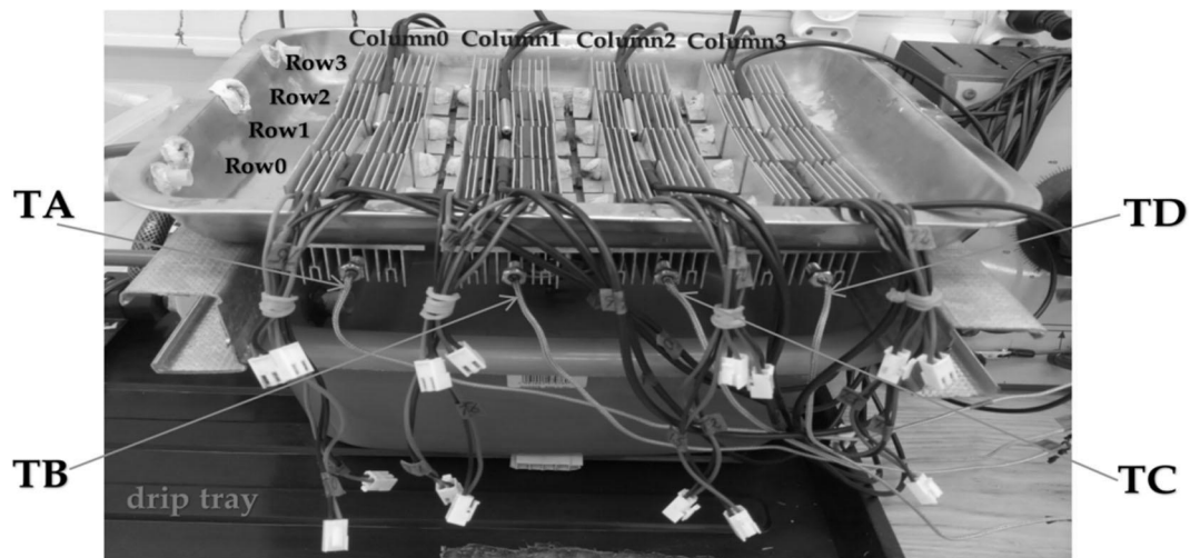
FIGURE 3 | Depiction of MAX6675 thermocouples TA, TB, TC, and TD, respectively inserted briefly inside the middle groove of the heatsink on Row0 TEHs (TEHs0–3) cold-side. During measurement at a particular voltage (12, 10, 8, 6, and 4 V) in succession; TA, TB, TC, and TD will be in turns moved to Row1, then Row2, and finally Row3 to measure all 16 TEHs heatsink cold-side temperature, before moving to the next voltage and the procedure repeated. By so doing, TA will only measure Column0 TEHs, TB will only measure Column1 TEHs, TC will only measure Column2 TEHs and TD will only measure Column3 TEHs. The x16 DS18B20 thermocouples are each permanently inserted inside the groove of the heatsink on the TEHs hot-side.
