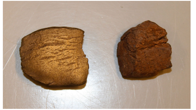
Fig. 3. Gold coated expanded schist sample (left) versus non-coated sample (right).
