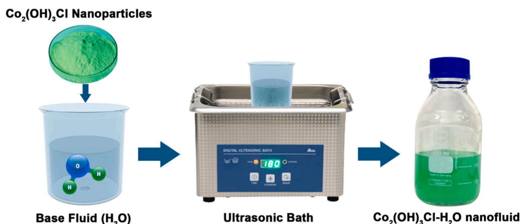
Fig. 1. \text{Co}_2(\text{OH})_3\text{Cl} - \text{H}_2\text{O} nanofluid preparation procedure.
