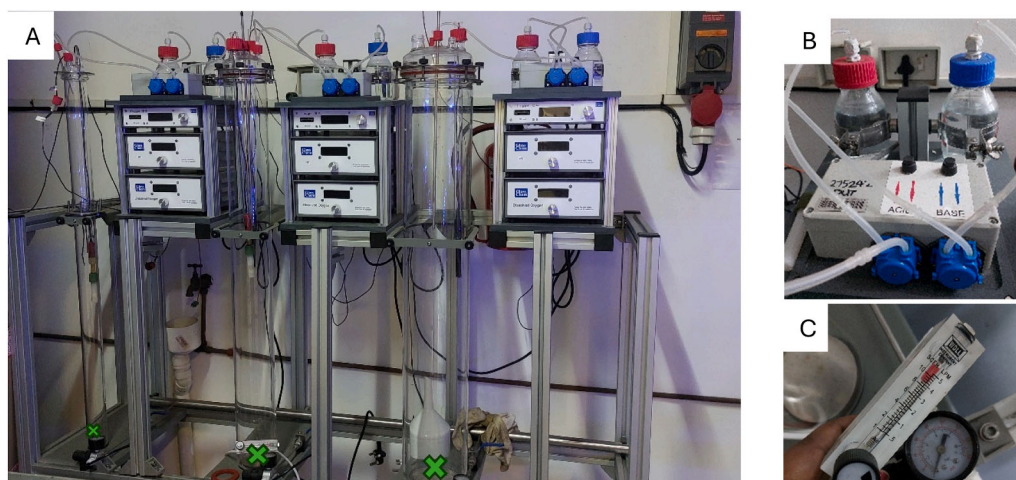
Fig. 2. Experimental setup of bubble column apparatus (C1, C2, C3), (b) automatic pH controller, and (c) flowmeter.
