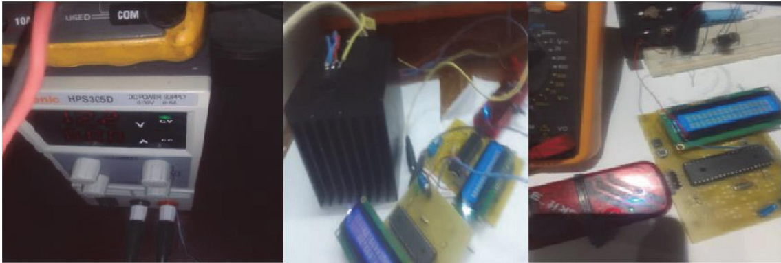
FIGURE 3: PCB prototype for the DCMFC-inverter integrated system. DCMFC, double-chamber microbial fuel cell.
