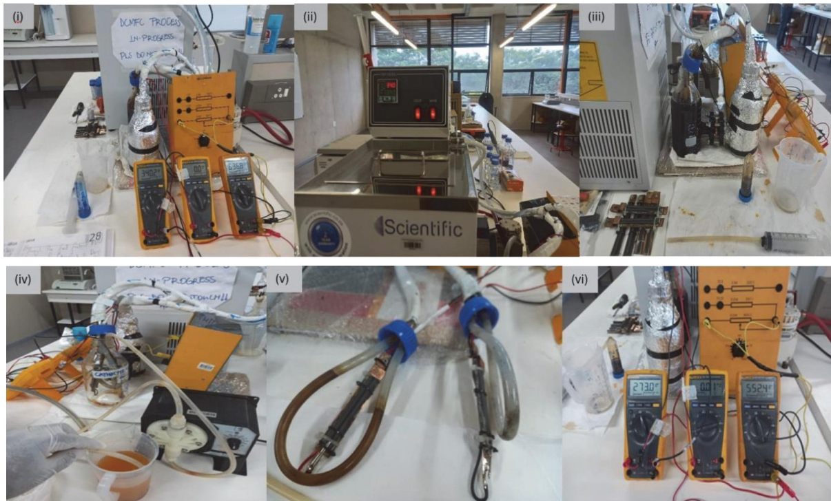
FIGURE 6: Real-time experimental set-up for the DCMFC, Shabangu et al. [52, 53]: (i) lab-set-up for the DCMFC in real-time, (ii) thermo-controller for controlled mesophilic-physcrophilic temperature, (iii) side view showing the cathodic medium and 0.1N as per optimized response output by the BBD-RSM design, (iv) the real-time fed-batch stop and subsequent start-up, (v) view the CCu-bi-electrode configuration with water circulating manifolds, and (vi) real-time optimized runs CCV values for the DCMFC. DCMFC, double-chamber microbial fuel cell; RSM, response surface methodology.
