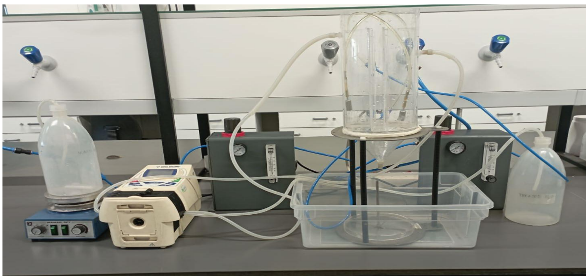
Figure 2. Photographic illustration of a column flotation.
