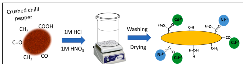
Fig. 1. Proposed preparation of AT-CP adsorbent.
