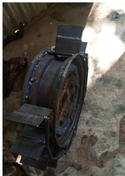
Figure 6. Challenge of replacement parts: original turbine replaced with improvised rim-welded turbine device (source V. Mwale).
