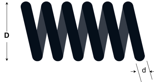
Fig. 6. Structure and parameters of tension or compression spring EDP.
