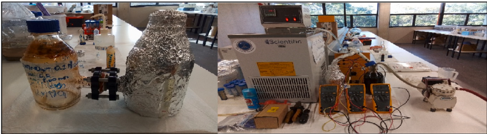
Fig. 3. MFC Experimental Set-up; Images of the start-up operation for the DCMFC system; component sections; aerator pump; DCMFC configuration chambers; Temperature controlling unit; Resistor box and water circulation set-up.
