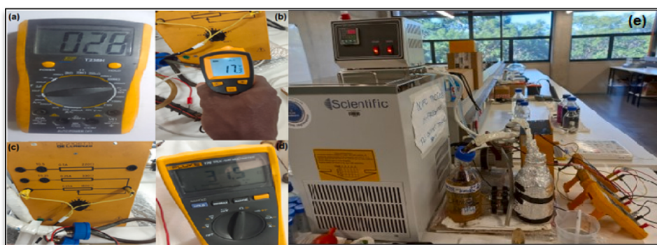
Fig. 6. Presents calibration test instrumentation (a) Infrared digital thermometer (b) Contact thermo-couple thermometer (c) Resistive load (DL2108T11) (d) Fluke digital multimeter (DMM) (e) Thermo-Scientific temperature controller for the DCMFC system.
