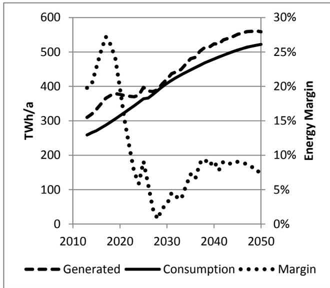
**Figure 6. Comparison of energy generated and consumed for Green Shoots scenario, and the energy margin**
