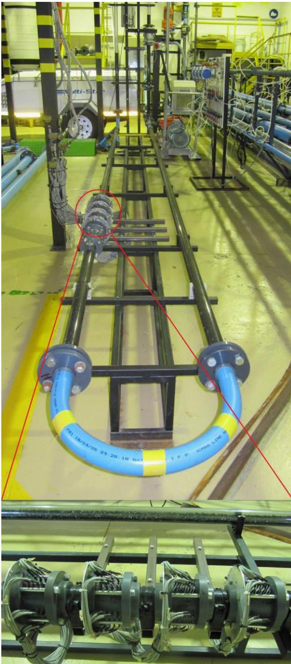
Fig. 2. FPRC pipe test loop with deposition probe spool pieces (ID 42.6 m) [17].
